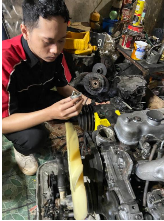
Gambar 3.3. Proses pengecekan Thermostat
