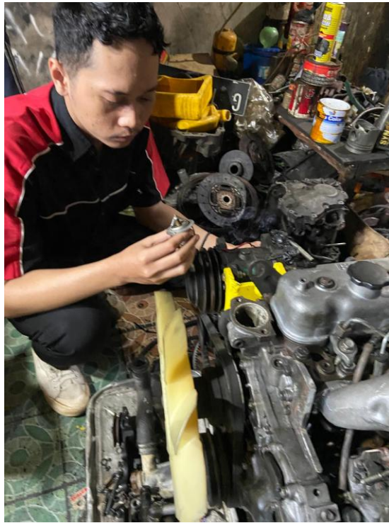
Gambar 3.3. Proses pengecekan Thermostat
