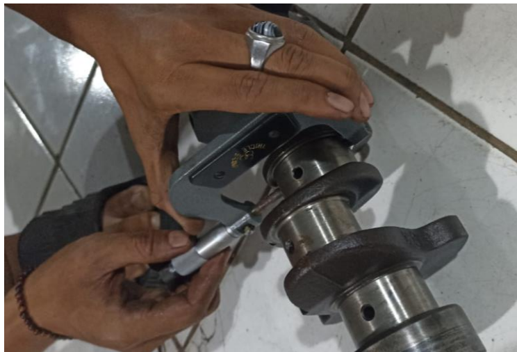
Gambar 18 Mengukur Diameter Crank Journal
