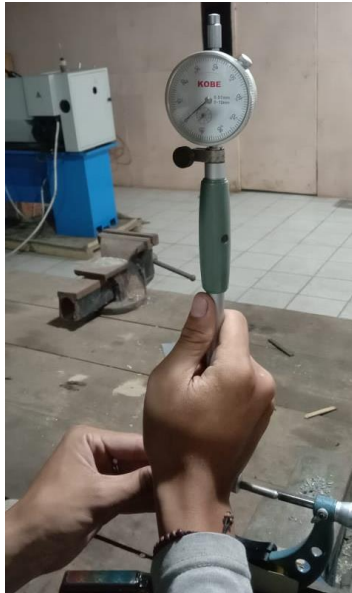
Gambar 13 Menyeting Dial Bore Guage
