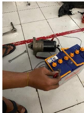
Gambar 17 pengujian pull in coil
