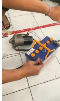
Gambar 18 pengujian hold in coil
