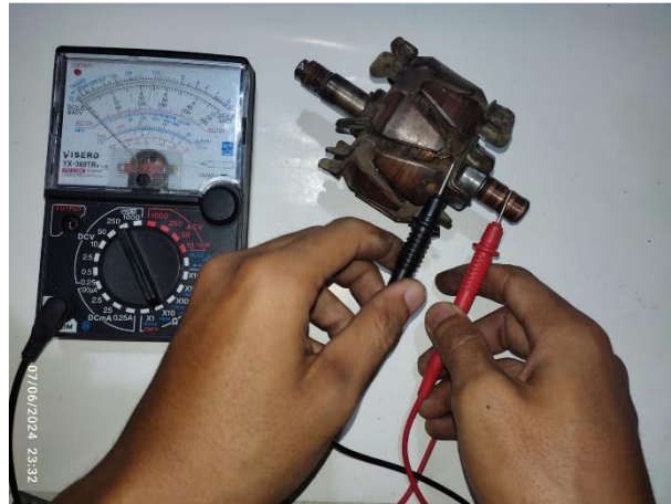
Gambar 10 Pemeriksaan Ground Rotor Coil
