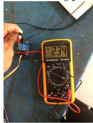
Gambar 4.8 Pengecekan Pin NO Relay
