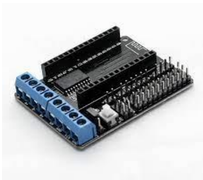
Gambar 3.2 Drive Shield NodeMcu 8266
