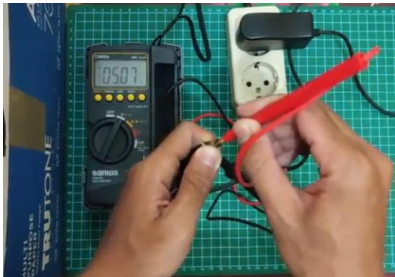
Gambar 4.0 Pengecekan Adaptor 5V
